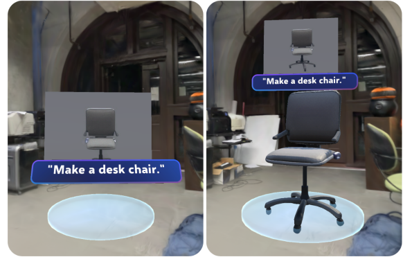
Figure 10: 3D and 2D Proxy Representations: (Left) New 3D proxy showing a low fidelity mesh preview (Right) Original 2D proxy representation with image preview
